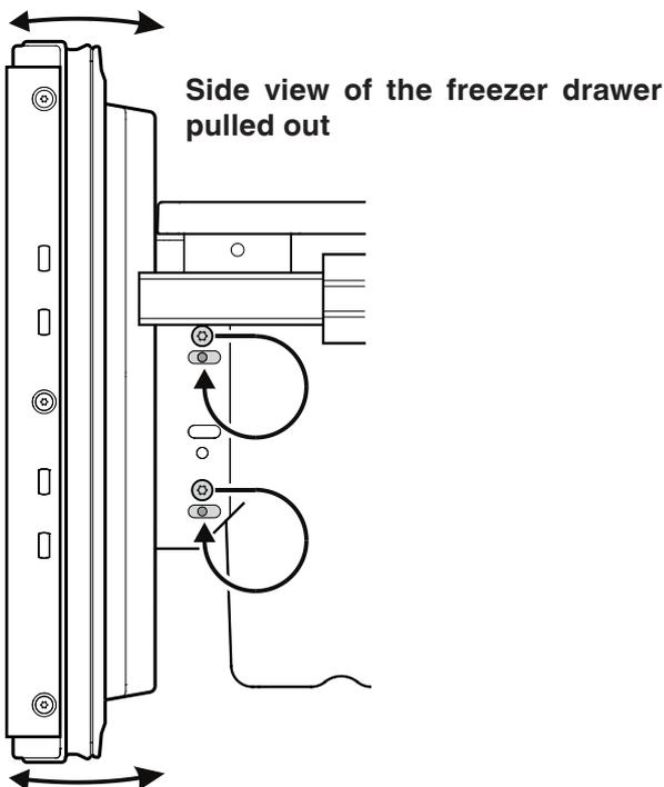
Unscrew the attachment brackets (3) from the freezer drawers. These attachment brackets will be mounted onto the freezer panels.
