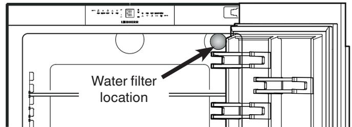
Replace the filter when the waterdrop symbol appears in the temperature display.
