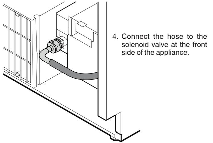
4. Connect the hose to the solenoid valve at the front side of the appliance.
