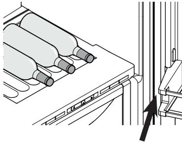
When storing tall bottles, the bottom door rack must be moved further up.
