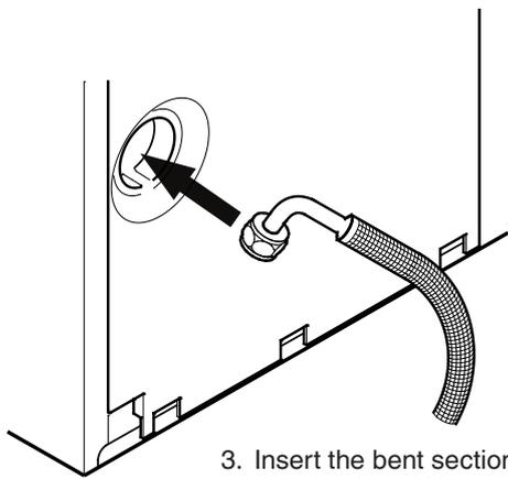
3. Insert the bent section of the hose through the opening at the rear of the appliance.
