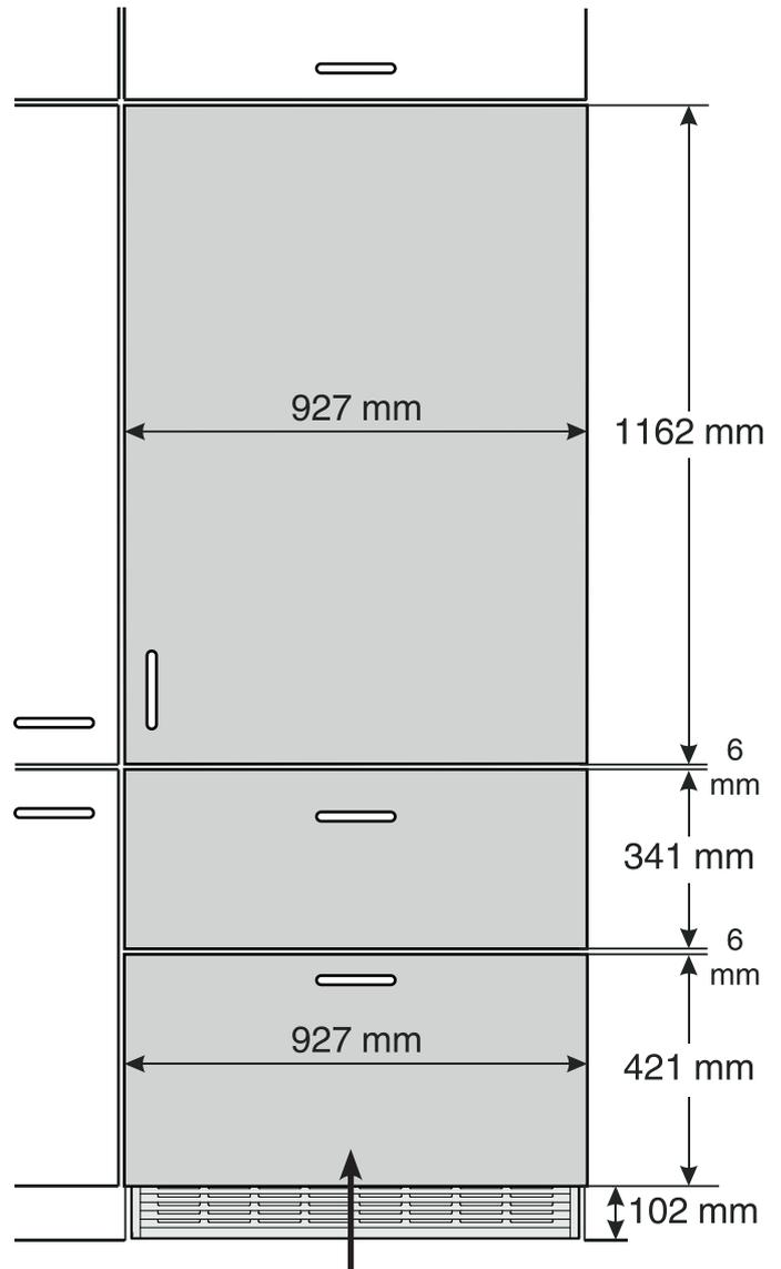
The height of this panel cannot be reduced for taller toe kicks as it will reveal structural elements of the appliance. Instead, install appliance on a platform and adjust the opening height to accommodate.
