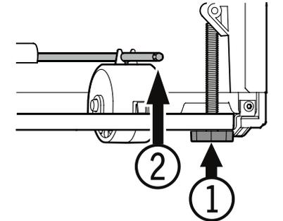
2. Adjust the height of the appliance at the rear by turning the adjusting bars (2).
